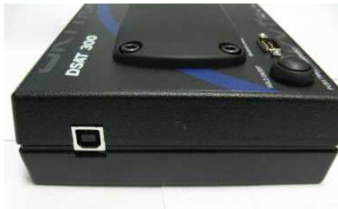
Figure 34 – Enclosure Assembly Gap
