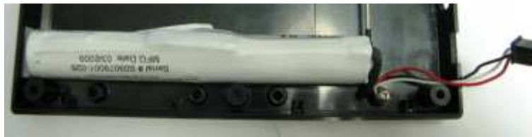
Figure 28 – Battery Tangent to Mounting Bosses
