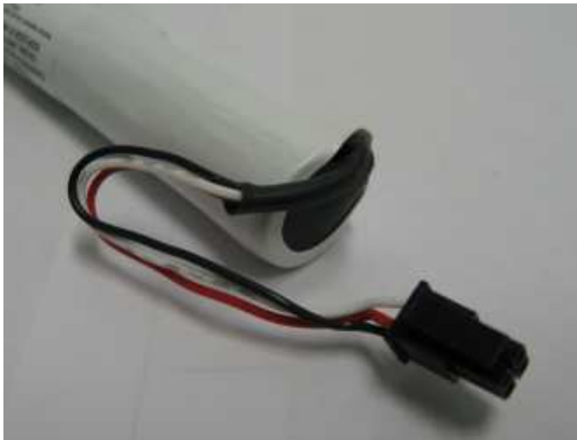
Figure 10 – Top Battery Cable Bends
