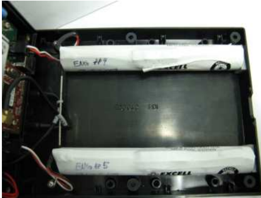
Figure 15 – Battery Installation Complete
