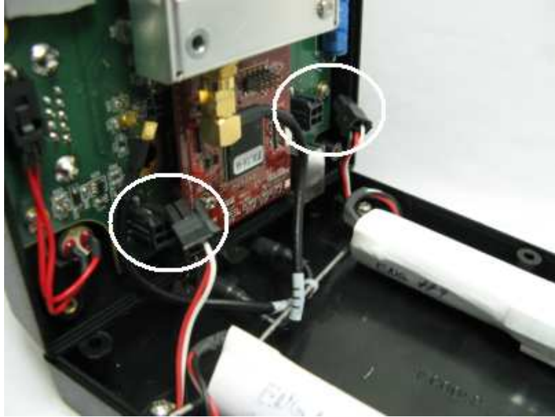
Figure 5 – Disconnecting the Batteries
