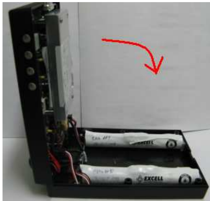
Figure 16 – Lowering the Enclosures
