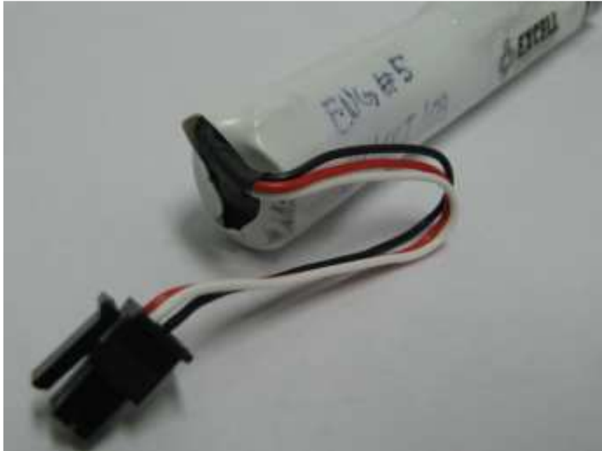
Figure 9 – Bottom Battery Cable Bends
