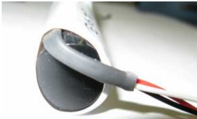
Figure 8 – Battery Cable Bend
