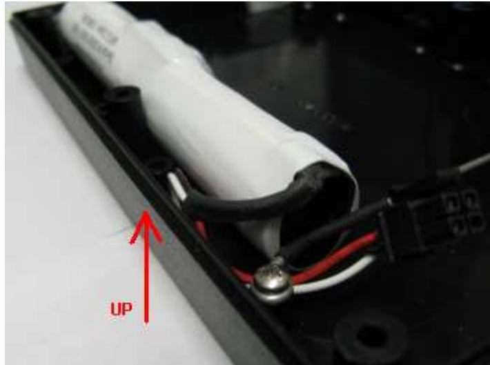
Figure 29– Battery Cable Orientation
