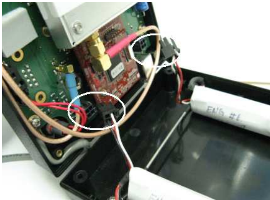
Figure 23 – Disconnecting the Batteries
