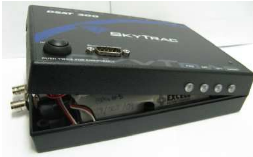
Figure 17 – Enclosure Pivoting at Right Side
