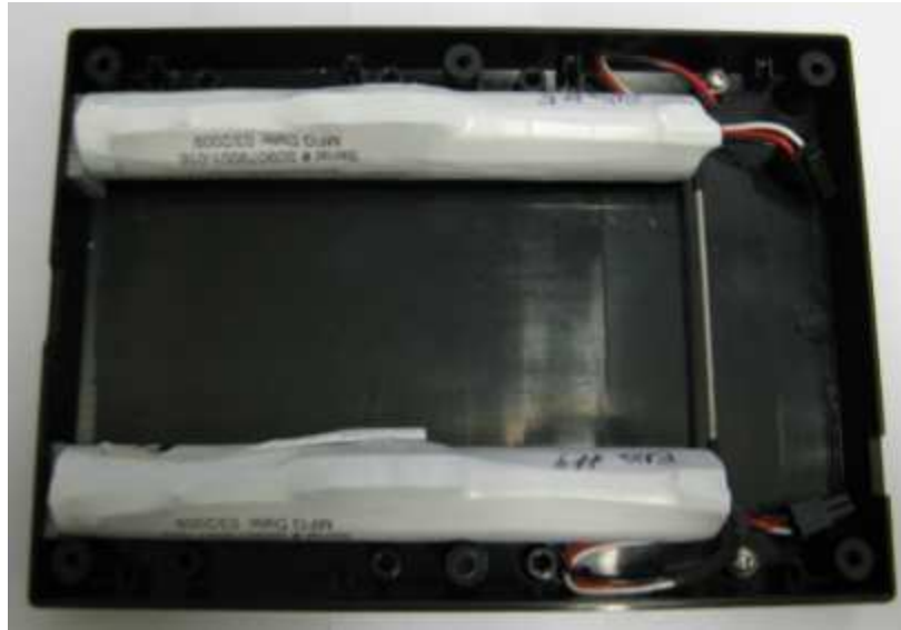
Figure 31 – Battery Installation Complete
